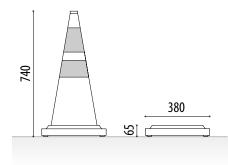
Moncayo model folding signaling cone 380x740 mm. Made of easy-folding orange waterproof reflective fabric with a rubber base.
