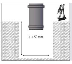
1. Perform a hole for the bollard installation. Preferably with diamond bit drill, if it is not possible to use jackhammer or rotary.
