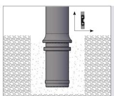
4. Level the bollard correctly.
