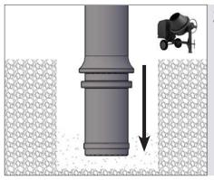
3. Introduce the bollard inside the hole and fill it with concrete.
