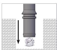
Put newsprint into the hollow bottom of the bollard in order to avoid concrete entry in the inside.
