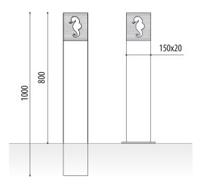
Aqua model bollard built with corten steel sheet with stainless steel top with marine motifs (starfish, seahorses, fish, dolphins, octopuses, whales,...).
