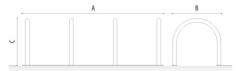
**Arra bicycle rack** made out of galvanised steel, or 304 or 316 stainless steel with 4, 5 or 6 round tube racks. 80x8 longitudinal lower base.
