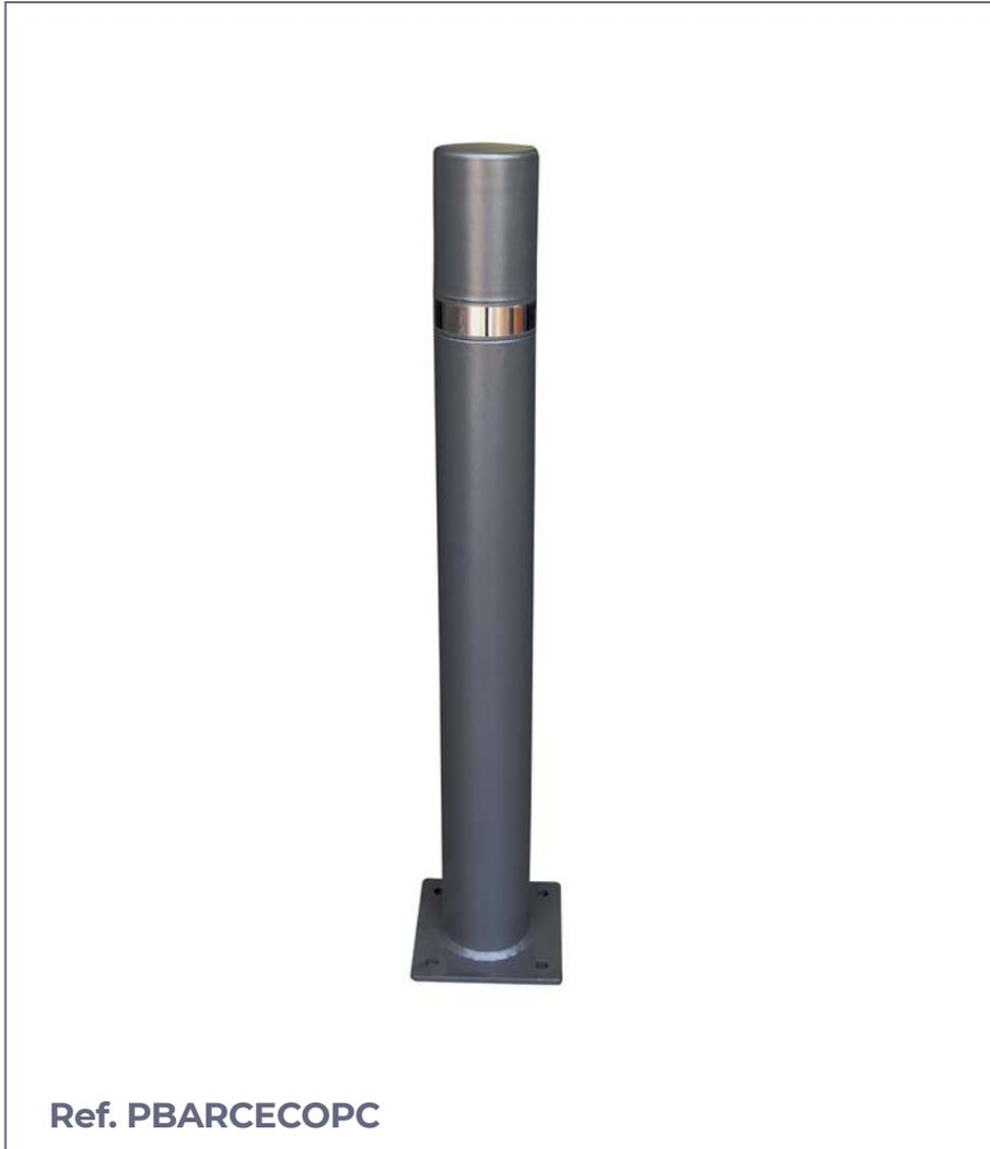
**Barceco bollard** made of iron tube with a diameter of  $\varnothing$  90 and 2.0 mm. of thickness. Overall height 800mm. With stainless steel ring at the top. Head with rounded edges avoiding possible damage to people.
