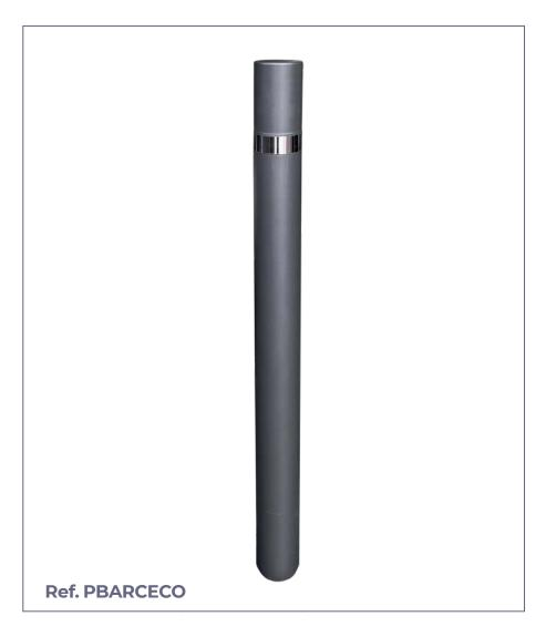
Barceco model bollard built with an iron tube with a diameter of ø 90 and 2.0 mm. of thickness. Total height 1000 mm. With stainless steel ring on the top. Head with rounded edges avoiding possible damage to people.
