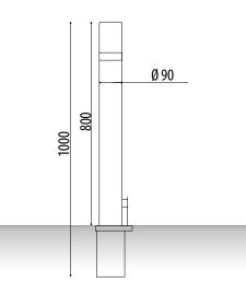
Removable Barceco bollard made of iron tube with a diameter of ø 90 and 2.0 mm. of thickness. Overall height 1000mm. With stainless steel ring at the top. Head with rounded edges avoiding possible damage to people.
