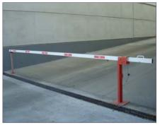
**Manual barrier model BM6** built with IPN 100 with mechanism for placing the aluminum pole, provided with locking system by manual lock pin and with gas piston to facilitate the opening and closing of the mechanisms.
