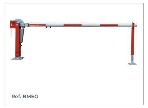
Manual barrier BMEG built with two 100x80x3 mm tubes. with mechanism for lodging the aluminum pole. Provided with a locking system by means of a lock. Two gas pistons to facilitate the maneuver of raising and lowering the barrier. Height-adjustable fixed support. Galvanized finish plus red lacquer. White lacquered aluminum pole with red stickers.
