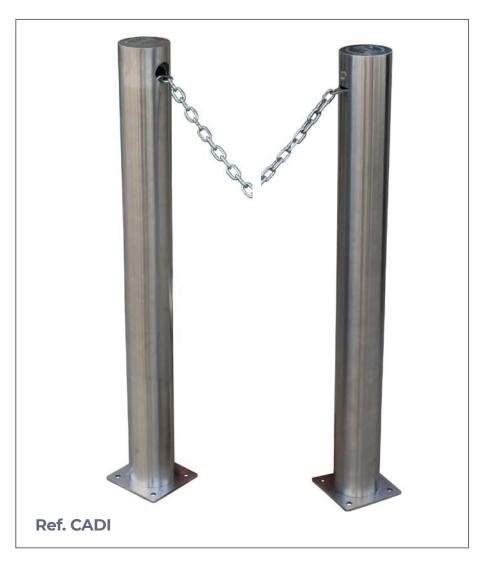
Cadi model manual chain bollard consisting of two ø 104 or 204 mm stainless steel bollards. (depending on the model) with a galvanized chain housed inside one of the bollards. Bollard with security lock that allows the chain to be collected inside the bollard.
