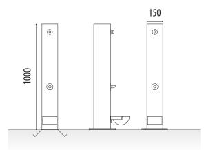
Canine model urban fountain in ovenlacquered iron for greater resistance to corrosion. Upper button and lower tap for filling the drinker.
