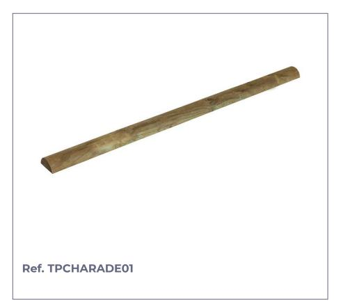
Charade wooden wheel stoppers of 1500 mm. long, built with class 4 autoclaved pine wood and fixed to the ground by embedding.
