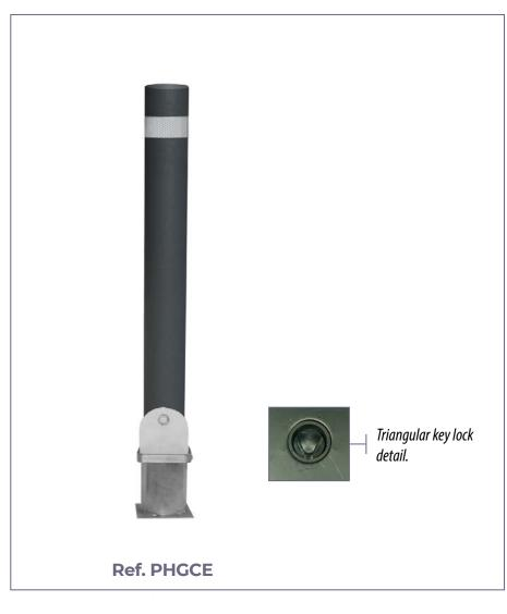
Removable cylinder model bollard, made of iron tube with a diameter of ø 95 or 220 mm. and 2.5mm. thick with reflective tape on the top improving its visibility. Total height of 1000 mm.
