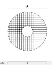
High-resistance circular rod tree made of 2 pieces of 30x30x2 mm rod. and ø 5mm. diameter.
