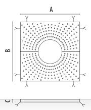
Concentrico tree grate built in 2 pieces of galvanized or corten sheet metal, in the form of a tray and reinforced with handrails. Includes angle frame with anchors to fix to the pavement.
