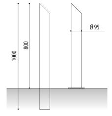
Bollard with flute-type upper cut, built with iron tube of diameter ø 95/200 mm. and 2,5 mm. of thickness.
