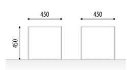
Cube reinforced concrete single-seat bench manufactured with only one block, resulting in a very heavy and robust bench, which is vandalresistant and requires virtually zero maintenance.
