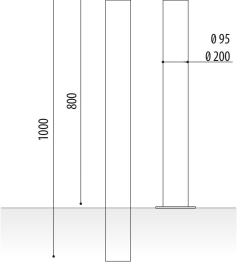
Dalo model bollard built with an iron tube with a diameter of ø 95 or 200 mm. and 2.5 mm. of thickness. With 8 mm stainless steel top cap.
