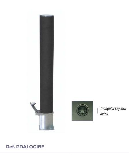
Dalo model removable bollard, built with iron tube of  $\emptyset$  95 or 200 mm. in diameter and 2.5 mm. of thickness. With 8 mm high stainless steel top cover.
