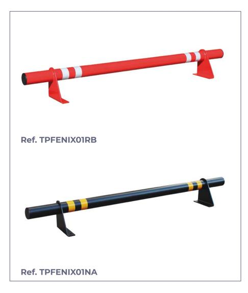
Fenix model iron wheel stopper of 1800 mm. long, built with iron tube diameter ø 80 mm. oven lacquered and 2 mm. of thickness.
