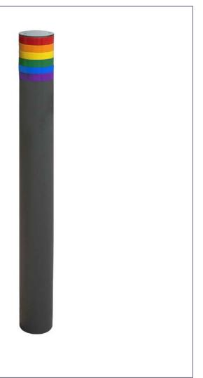
Flag model bollard built with ø 95 and 2.5 mm diameter iron tube. of thickness. Total height 990 mm. The colored rings are interchangeable according to customer needs.
