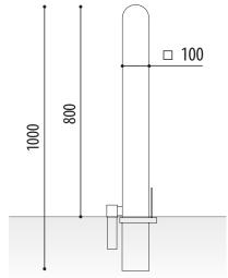
Removable anti-moon security bollard model Gray 100 of great robustness with security lock to anchor to the ground.
