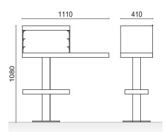
Urban Grill barbecue made from corten sheet with different thicknesses. Main body made of 10 mm sheet metal. and 5 mm top hinged lid. ø100x3 mm tube. with square lower plate of 350x350 mm. to fix to the ground.
