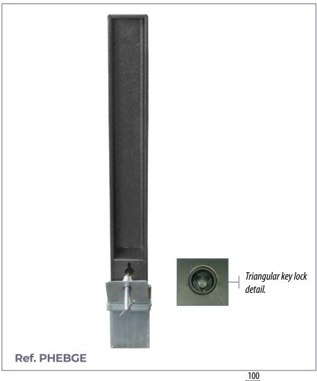
Removable HEB bollard built with 100x100 mm iron beam. Overall height 1000mm. Galvanized ground-anchoring base for bollard housing with universal lock.
