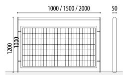
Hera model modular urban railing built in galvanized steel with round tube handrail, plate uprights and mesh housed inside.
