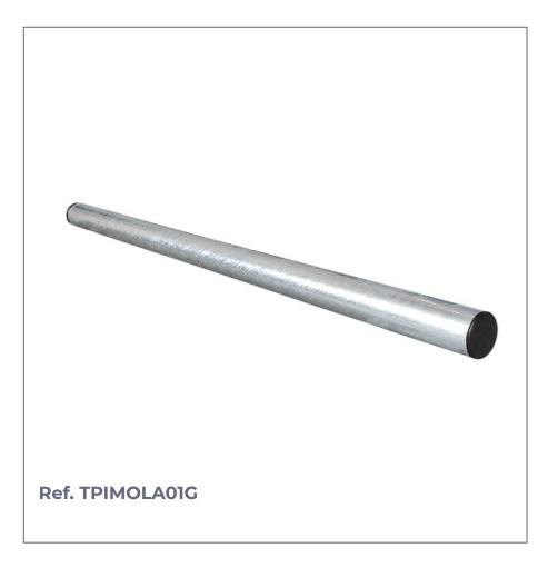
Imola model iron wheel stopper 2000 mm. long, built with iron tube diameter ø 80 mm. oven lacquered and 2 mm. of thickness. ground fixing by corrugated rod.
