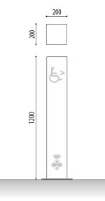
**Info model corten steel luminous bollard with low consumption LEDs,** built with 200x2000 mm corten steel tube.
