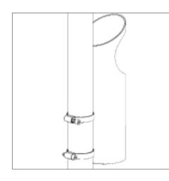
Fix both ashtray and flanges on the litter bin post, close the flanges and tighten the screw.
