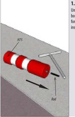
**Unscrew HA75** bollard's female anchor for subsequent ground installation.
