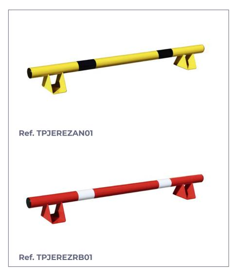
Jerez model iron wheel stopper 1800 mm long, built with iron tube diameter ø 80 mm. oven lacquered and 2 mm. of thickness.
