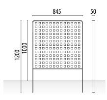
King model modular urban railing built with handrails and perforated sheet metal inside.
