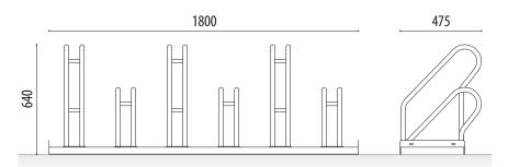
Modul bike parking formed by only one piece in galvanised steel, which can store up to 6 bikes parked in an alternate, bidirectional row, with a rectangular base of 375x1800 mm.
