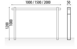
Olimpo model modular urban railing built with uprights similar in design to the Olimpo bollard (rectangle-shaped handrail with central iron reinforcement).
