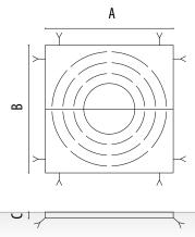
Onda model tree pit built in 2 pieces of galvanized or corten sheet metal, in the form of a tray and reinforced with handrails. Includes anchor frame to fix to the pavement.
