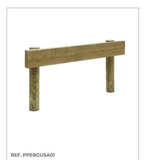
Pergusa vehicles stopper of 2000 mm. long, built with class 4 autoclaved pine wood and fixed to the ground by embedding.
