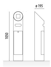
Circular bollard ashtray for outdoor model Pilce with an innovative design. Highly impact resistant ashtray with a large capacity for butts inside (9 litres).
