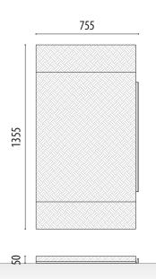
Plastrong model plastic trench cover walkway, ideal for covering temporary holes in construction sites.
