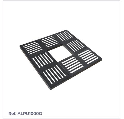
**Puzzle tree grate** built in 4 rectangular pieces of galvanized or corten sheet metal, in the shape of a tray and reinforced with handrails. Includes angle frame with anchors to fix to the pavement.
