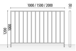
Queen model modular urban railing built with a folded rectangular tube frame and round tube bars.
