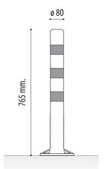
Road delimiter flexible post made of highly flexible polyurethane plastic. In case of impact the pole returns to its original position. Reflectorized post with three high visibility reflective tapes. In the upper part it has a 26 mm hole for fixing accessories. Bollard / post Ideal for delimiting roads, streets, private spaces, use in industrial spaces, etc.
