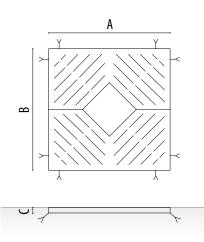
Rombo tree grate built in 2 pieces of galvanized or corten sheet metal, in the form of a tray and reinforced with handrails. Includes angle frame with anchors to fix to the pavement.
