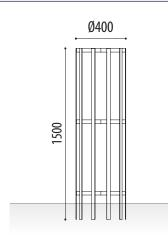
Sauce tree guard manufactured with horizontal bent plates and vertical plates. Made out of primed and lacquered steel, available in different colours. It is supplied in 2 pieces to join by means of anchors. Tree guard for outdoor installation ideal to protect urban spaces.
