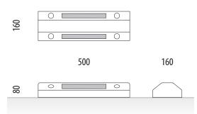
Silver wheel stopper made of polypropylene plastic with yellow reflective tape with microspheres measuring 500x160x80 mm.
