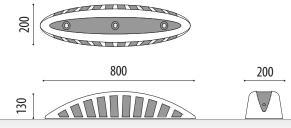
Snake model bike lane separator made with recycled material in 1 single piece measuring 800x200x130 mm. Black color and paint with white reflective microsphere.
