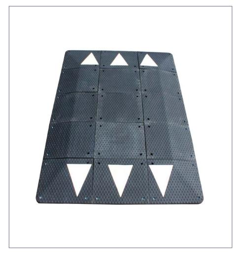
Berlin Mitte model prefabricated rubber cushion for urban roads. The cushion is an elevation implanted in the middle of the road that constitutes an obstacle depending on the distance of the wheels of the same axle of the vehicle that allows buses and other heavy vehicles not to be affected by it, since the separation between wheels It is wider than the height of the Berlin cushion.
