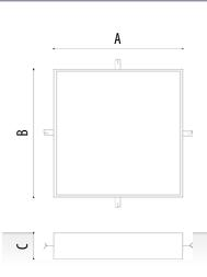
Square or rectangular tree frame to define the space of land that the tree needs for its growth. It is manufactured with galvanized sheet or corten sheet.
