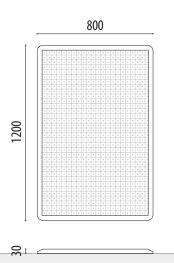
Swiper model trench cover ideal for covering holes and temporary trenches on construction sites.
