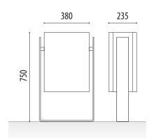
**Tali urban litter bin** with elaborate design, suitable for all types of settings and environments due to its diverse material combinations (ordinary, wathering and stainless steel).
