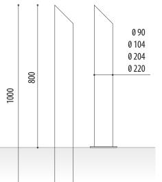
Tecor stainless steel bollard with flute-like cut, manufactured with AISI 304 stainless steel tube with a diameter of 90, 104, 204 or 224 mm. With matte or glossy ring.
