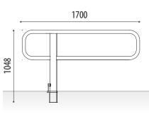
Track model iron manual road closure barrier. with removable base that allows, by means of a key on the base, to have the barrier in two positions: open or closed.
